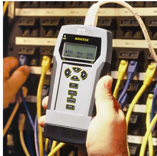
Picture 4: PING an IP device with NAVITEK
